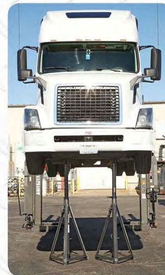
Model 9-THR High-Rise vehicle support stands working with Gray's Patented Wireless Portable Lift System
