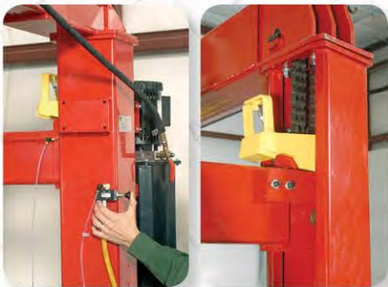
Single point, pneumatic locking mechanism & simultaneous lock release from one location
